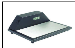
Fig. 2. UVP Heater: Temperature Stability for Western blots development.
