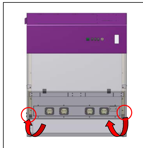
UV2 PCR Cabinet and Workstation. Airflow into and out of the UV Air Circulator
