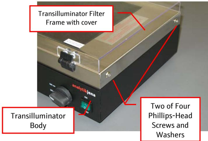
5. Using the pliers, remove the **securing nut** securing the selector switch to the transilluminator body.
