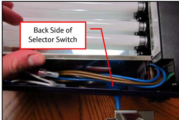
9. **Note:** Prior to completing this step, make a note of the location of the transilluminator selector switch wiring on the gray wiring junction block.
