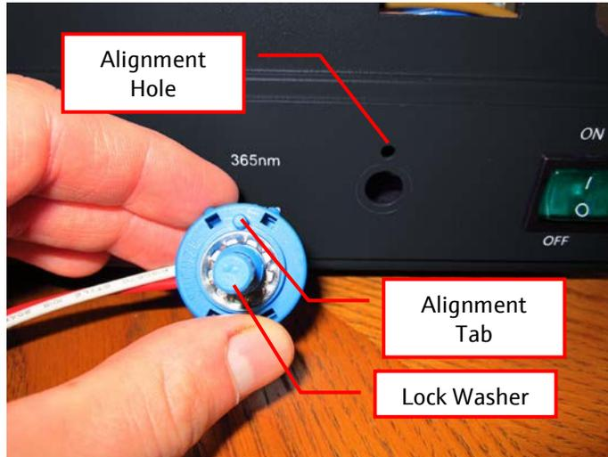
2. Place the **lock washer** over the shank of the replacement selector switch.
