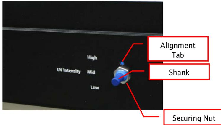
5. Without the selector switch knob installed, use your fingers to rotate the selector switch shank to the lowest position (in this case, to the "302nm" position).
