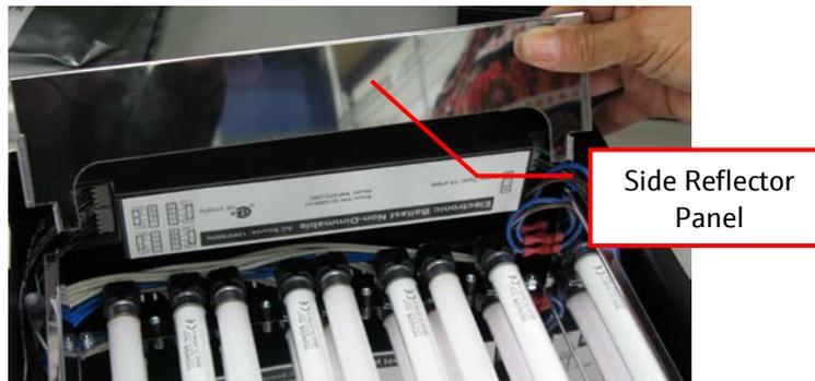
7. Pulling straight up, remove the two side reflector panels from inside the transilluminator.
