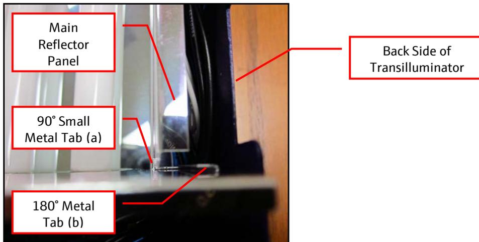
11. As the edges of the side reflector panels are sharp, ensure that all wiring is moved out of the way during installation of the side reflector panels to avoid cutting into the sheathing of the wiring. Slide the side reflector panels into place until the top edges of the reflector panels are flush with the top edges of the main reflector panel.
