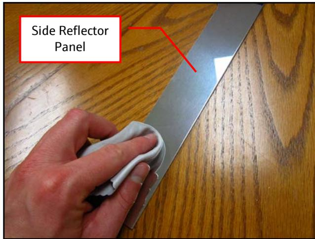
10. The side reflector panels must be aligned with the **main reflector panel** during reinstallation.
