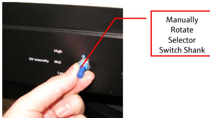
6. The selector switch knob does not have a groove or flat surface to align on the selector switch shank, so it is necessary to visually align the white indicator line on the knob with the desired indicator position on the face of the transilluminator.
