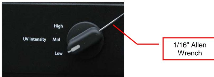
3. While firmly holding the transilluminator housing, pull forward on the knob to remove it from the selector switch shank. *Note: This process may require a fair amount of force as the knob fits snugly over the shank.*
