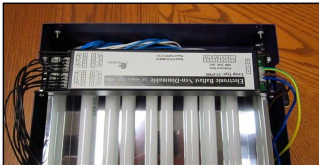
7. Place the new ballast next to the old ballast, also atop the fixed reflector panels, in the same orientation as the old ballast.
