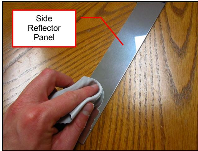
4. The side reflector panels must be aligned with the main reflector panel during reinstallation.
