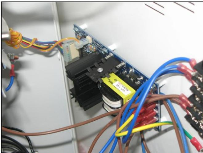
3. Unplug all wires from the old control board, noting the position of each. **NOTE:** All wiring must be reconnected in the same positions.
