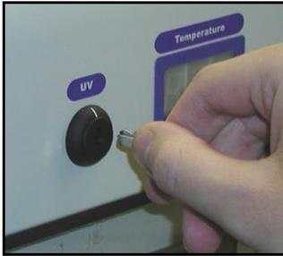
*Insert the UV key to operate the shortwave UV. Remove the key after using the UV to avoid accidental exposure of samples during incubation.*
