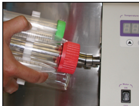
Installing the carousel
