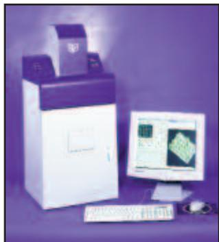
*BioSpectrum Imaging System* connects to a computer installed with VisionWorksLS Analysis Software. Imaging applications include chemiluminescence, fluorescence and colorimetric. For plant/live animal studies, ask about the BioSpectrum 600 which includes the OptiChem HR Camera for deeper cooling, for higher sensitivity and extended integration times.
